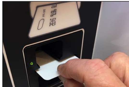
Figure 4: TT8800 OPT Inserting a Reader Cleaning Card
