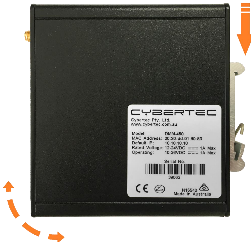
Figure 27: T20 CMM Module Replacement
