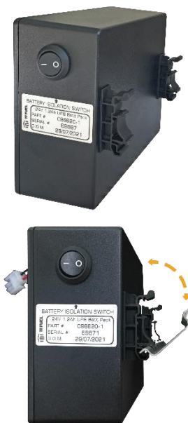
Figure 29: UPS Battery Replacement
