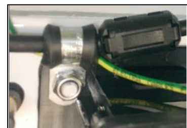
Figure 22: TT8900 OPT Anti-Vibration Nuts
